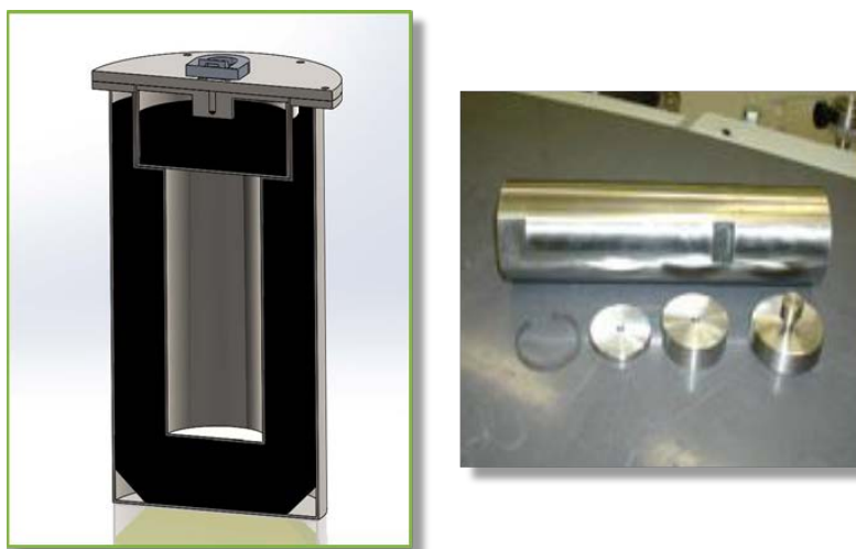
Fig. 1. Proposed Type A packaging for irradiated Ac-225: Type A packaging concept on left; Model II special form capsule on right.
